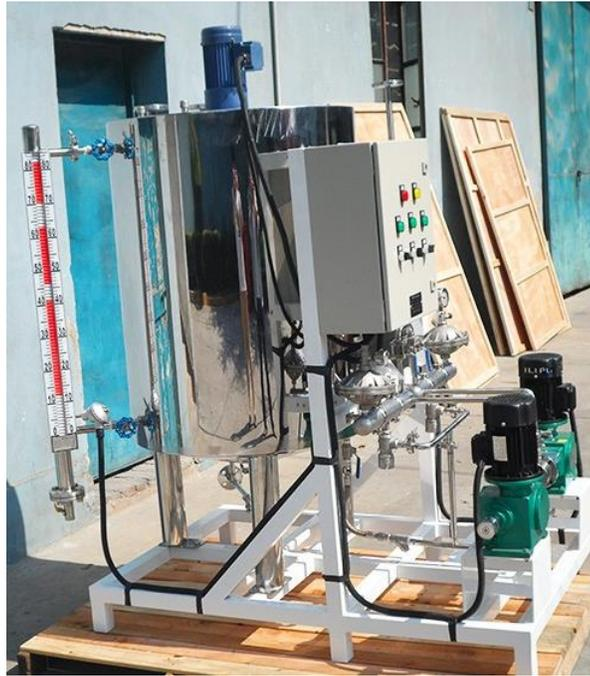
**Nota.** Se muestra un tanque de mezclado de acero inoxidable fabricado por la marca Amixer. Tomado de: [94] Alibaba.com, “20l 30l 50l 200l 500l 1000l Stainless Steel Liquid Mixing Tank - Buy Mixing Tank 3000 L Agitator, Mixing Tank 20l, 200 Liter Mixing Tank,” 2021. [Online]. Available: [https://www.alibaba.com/product-detail/20L-30L-50L-200L-500L-1000L\\_1600235862236.html](https://www.alibaba.com/product-detail/20L-30L-50L-200L-500L-1000L_1600235862236.html).
