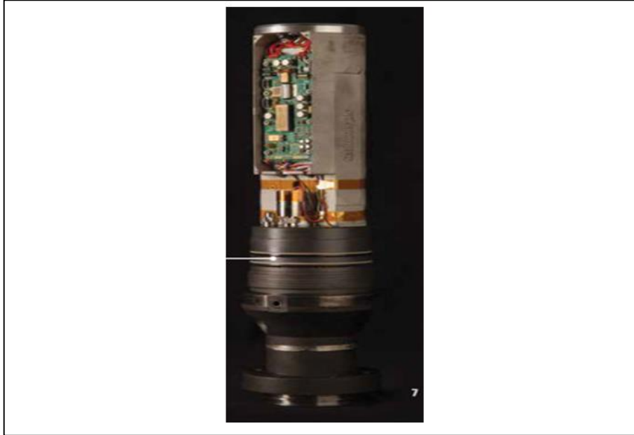
Figura 19. Phoenix xt150 downhole monitoring system
