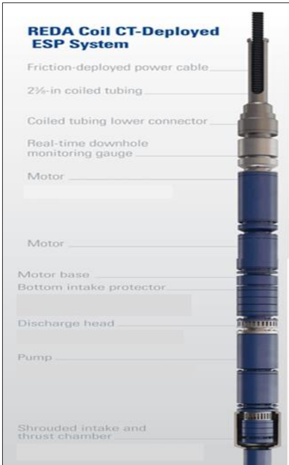
Figura 20. Partes de Reda Coil CT-Deployed ESP System
