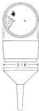
Figure 962.09B—Modified California State Büchner funnel, 2-piece polypropylene plastic, covered with 200-mesh screen, A, heat-sealed to edge of filtering surface.
