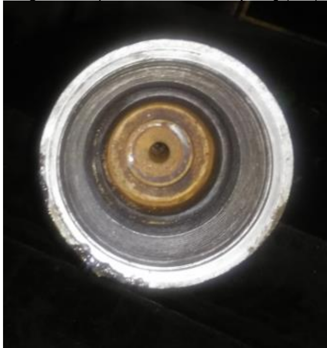
Figura 8. Tope herramienta Sand jetting (Box)
