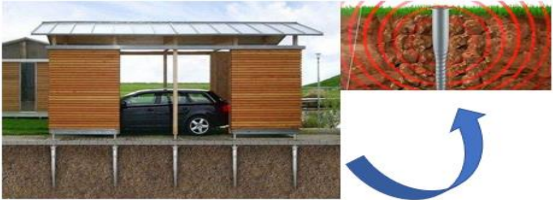
Figura 10. Ground Screw Foundations
